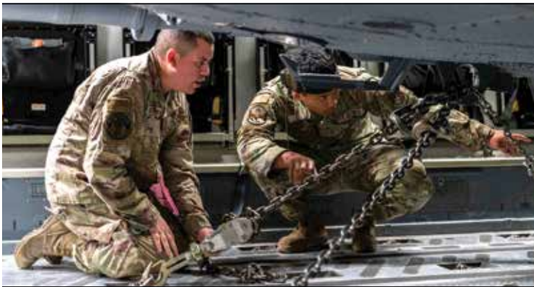
U.S. Air Force Airmen with the 33rd Helicopter Maintenance Unit and 718th Aircraft Maintenance Unit rig a towing bar to an HH-60W Jolly Green II at Kadena Air Base, Japan, Jan. 26, 2024.
