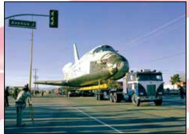
March 8, 1979: Space Shuttle Columbia arrived on a trailer after a 38-mile journey from the Rockwell International plant in Palmdale, Calif., through Lancaster then on to Edwards AFB. The first step in its travels toward space was taken at five to 10 mph. The orbital vehicle was delivered to NASA's Dryden Flight Research Facility to be mated with its Boeing 747 carrier aircraft.
