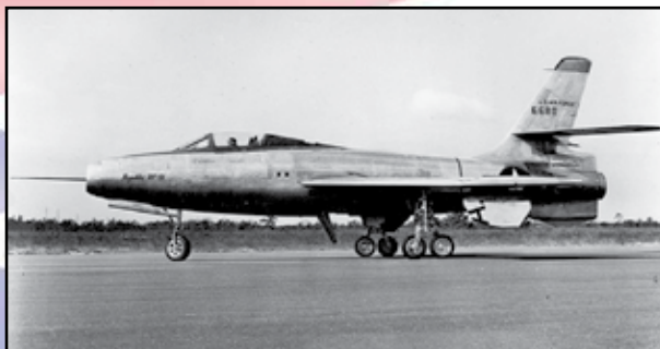
May 9, 1949: The initial flight of Republic's rocket-assisted jet fighter, the XF-91 Thunderceptor, took place piloted by Carl Bellingier. The aircraft was unusual in a number of respects. Its swept back wings were wider and thicker at the tip than the root; its dual-wheel landing gear retracted outward; and it carried an auxiliary jet motor at the base of its tail.
