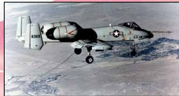
May 10, 1972: Fairchild Republic's YA-10A Thunderbolt II made its first flight, flown by company chief test pilot Howard "Sam" Nelson, in Farmingdale, N.Y. The twin-engine, twin-tailed ground attack aircraft was designed around the General Electric GAU-8 Avenger 30mm rotary cannon.
