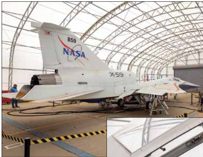
NASA photographs by Garry Tice NASA's X-59 quiet supersonic research aircraft is seen during its "aluminum bird" systems testing at Lockheed Martin's Skunk Works facility in Palmdale, Calif. The test verified how the aircraft's hardware and software work together, responding to pilot inputs and handling injected system failures.
