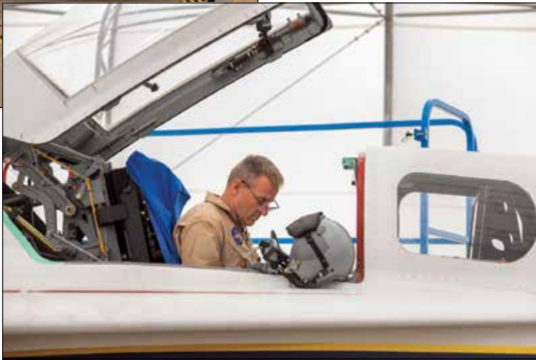
NASA photographs by Garry Tice NASA's X-59 quiet supersonic research aircraft is seen during its "aluminum bird" systems testing at Lockheed Martin's Skunk Works facility in Palmdale, Calif. The test verified how the aircraft's hardware and software work together, responding to pilot inputs and handling injected system failures.
