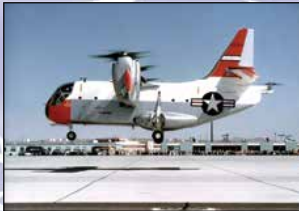
July 9, 1965: The tilt-wing XC-142A vertical/short takeoff and landing aircraft arrived at Edwards Air Force Base, Calif., for Category II testing following a two-day flight from the Ling-Temco-Vought plant in Dallas, Texas. The flight was the first long distance hop of a V/STOL aircraft. The XC-142A was an experimental four-engine propeller transport in which the engines and wings tilted in flight to transition between vertical and horizontal flight.
