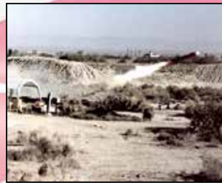
July 12, 1997: A Northrop Grumman crew launched a BQM-74 Chukar RPM from South Base at Edwards Air Force Base, Calif., to test its new JATO unit. The jet propelled drone was designed as a high-speed aerial target, and had also been used as a decoy over hostile territory.
