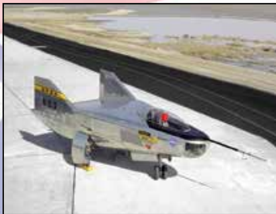
July 12, 1966: The Northrop M2-F2 heavyweight lifting body made its first flight at NASA's Dryden (now Armstrong) Flight Research Facility at Edwards, Calif., with test pilot Milt Thompson. The same B-52 used to air launch the famed X-15 rocket research aircraft was modified to also carry the lifting bodies. Thompson was dropped from the B-52's wing pylon mount at an altitude of 45,000 feet on that maiden glide flight. The M2-F2 weighed 4,620 pounds, was 22 feet long, and had a width of about 10 feet.
