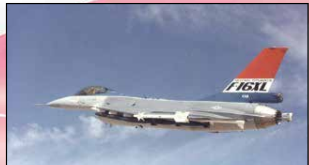
July 20, 1982: The first flight of the F-16XL took place. General Dynamics modified a FSD F-16 to answer a U.S. Air Force requirement for a dual-role, longer-range fighter to support future air combat requirements. The F-16XL featured a cambered, cranked-delta wing with a sharp leading-edge sweep with twice the area of the original wing.
