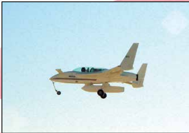
July 21, 2001: The XCOR EZ-Rocket, flown by Dick Rutan, made its first flight. The EX-Rocket was a test platform for the XCOR XR-4A3 rocket propulsion system. The airplane was a modified Rutan Long-EZ, with the propeller replaced by first one, then later a pair of pressure-fed regeneratively cooled liquid-fueled rocket engines and an underslung fuel tank. The engines were restartable in flight, and were contained within Kevlar armor shielding. The EZ-Rocket was registered as an experimental aircraft.
