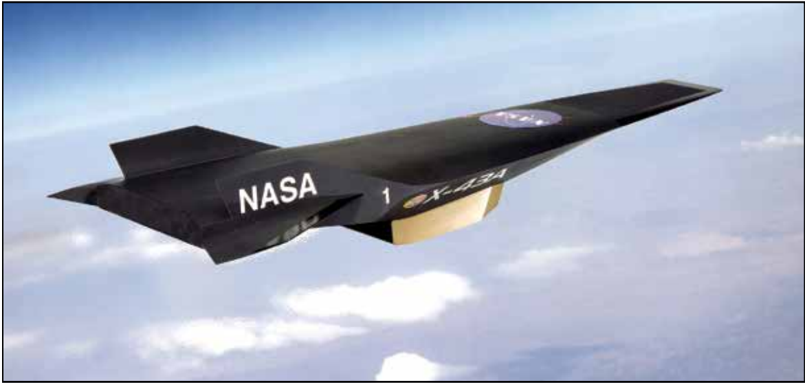
NASA image Artist's concept of X-43A with scramjet attached to the underside.
