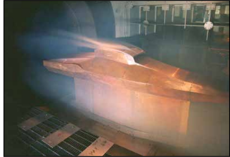
NASA photograph by Jeff Caplan A full-scale model of the X-43 plane in Langley's 8-foot, high-temperature wind tunnel.
