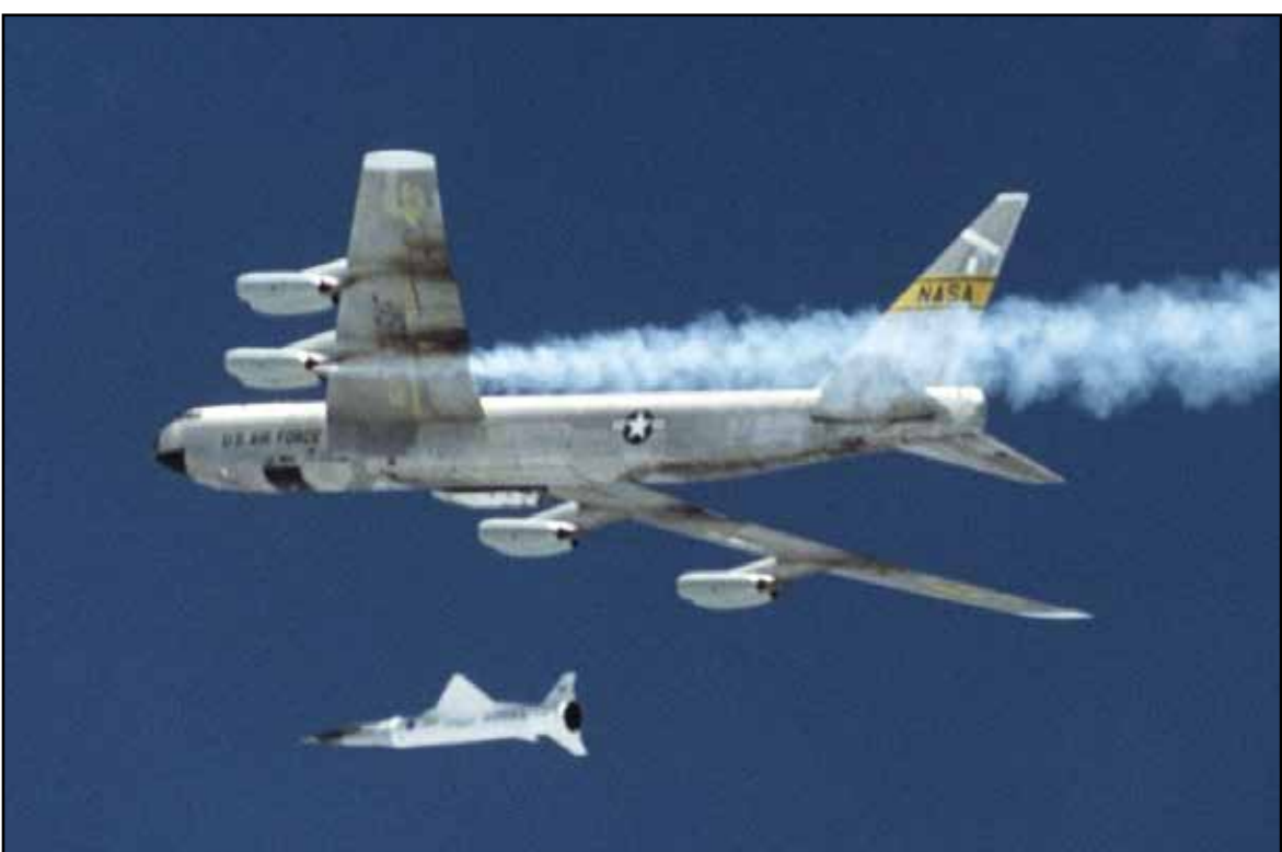
NASA photograph A NASA NB-52 Stratofortress with a X-43 Scramjet (modified Pegasus rocket).
