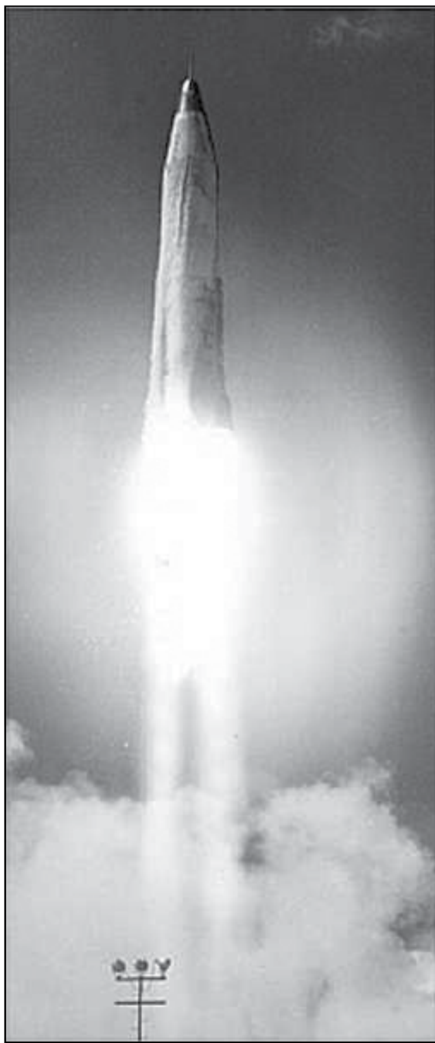
The Convair XSM-16A (later X-11) was the first testbed for what became the Atlas missile. Later the Convair X-12 became a second, more advanced testbed. A total of 12 X-11's were built and tested. The first three were involved in static tests only. X-11 Number 4 and 6, were destroyed in launch accidents. All others performed successful test flights. The test series began on June 11, 1957 and ended on June 3, 1958.
