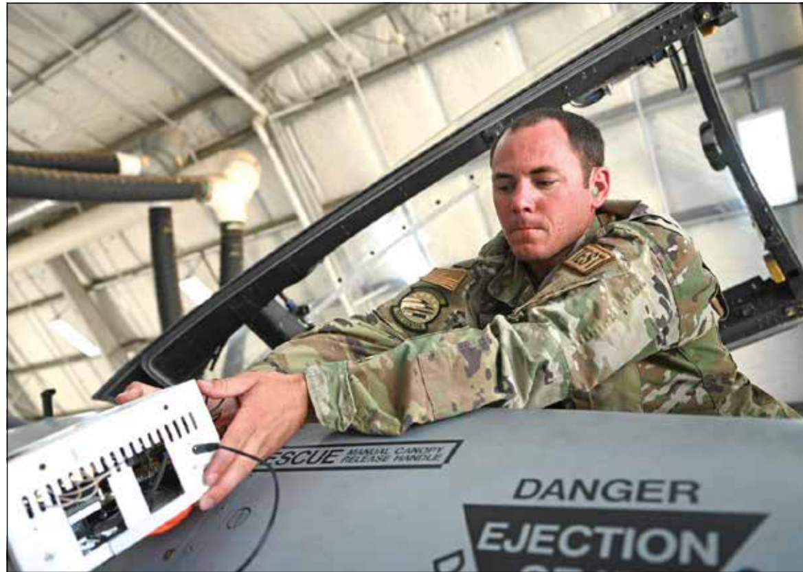
U.S. Air Force Staff Sgt. Tyler Sanders, Air National Guard Air Force Reserve Command Test Center avionics technician, pulls a Portable Automated Test Station into the cockpit of an A-10C Thunderbolt II aircraft at Davis-Monthan Air Force Base, Arizona, June 29, 2023. Sanders tested the wireless range by placing the PATS in different locations around the A-10.
