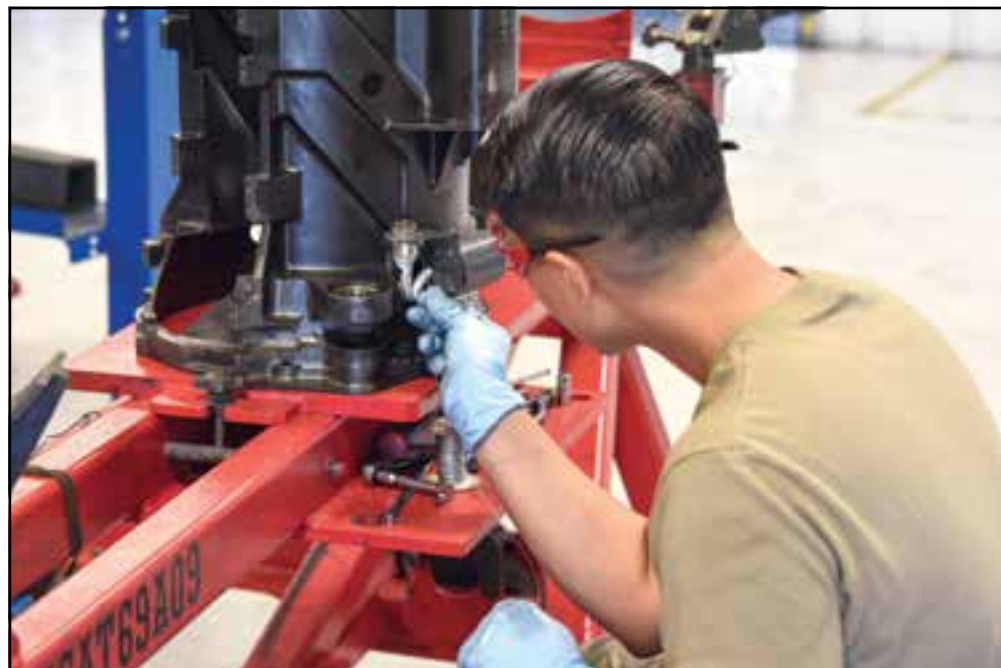
U.S. Air Force Staff Sgt. Joanna Garcia, 355th Munitions Squadron armament munitions supervisor, is safety wiring the GAU-8 Avenger 30mm auto cannon's electrical safety solenoid at Davis-Monthan Air Force Base, Arizona, May 24, 2022. This is done while the rebuild process for the gun is underway and ensures the electrical connector remains secure during firing sequences.
