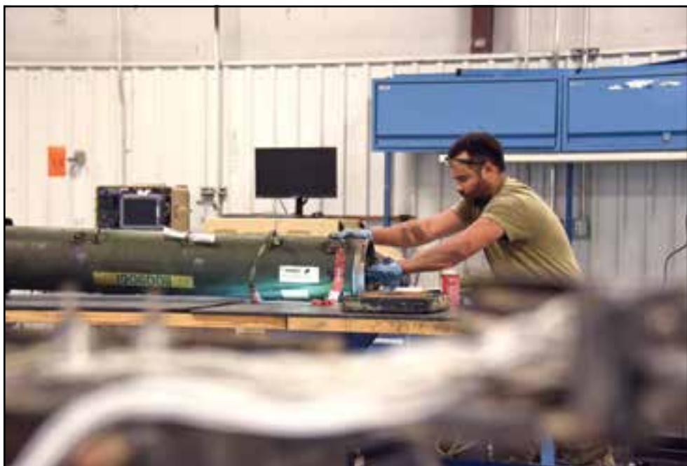
U.S. Air Force Staff Sgt. Joseph Clark, 355th Munitions Squadron armament munitions supervisor, cleans the firing contacts on a LAU-131 rocket pod while completing a 30-day storage inspection at Davis-Monthan Air Force Base, Arizona, May 24, 2022. Having clean firing contacts is essential to ensuring 2.75 inch rockets ignite and release when the fire signal is given.
