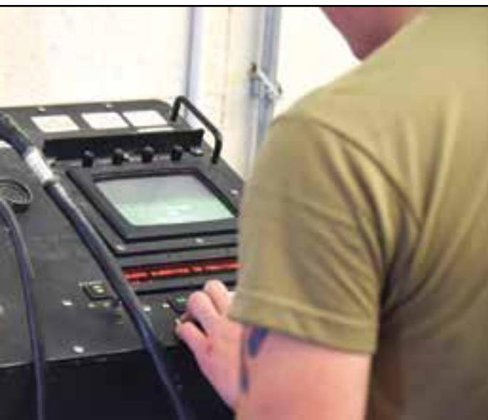
U.S. Air Force Airman Devin Aaronson, 355th Munitions Squadron precision maintenance technician, recalibrates a missile's guidance section at Davis-Monthan Air Force Base, Arizona, May 24, 2022. This allows Aaronson to align the crosshairs and lock onto targets in order to diagnose any malfunctions.
