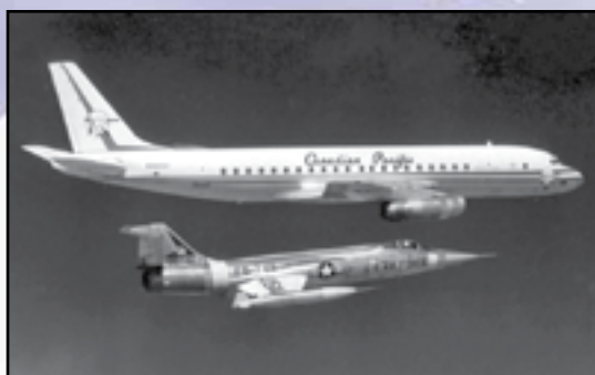
Aug. 21, 1961: A Canadian Pacific Douglas DC-8 commercial airliner broke the sound barrier — the first time a civil airliner had done so. The Douglas DC-8-3 climbed to 50,090 feet near Edwards Air Force Base, Calif. Placing the DC-8 into a dive, it reached Mach 1.012 while descending through 41,088 feet. The airliner maintained this supersonic speed for 16 seconds.
