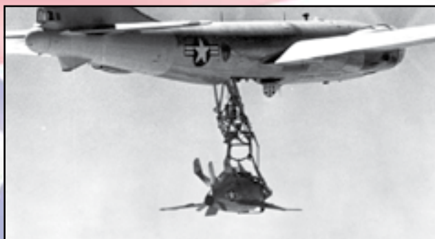
Aug. 23, 1948: The McDonnell XF-85 Goblin parasite fighter made its first flight. On this flight, McDonnell test pilot Edwin F. Schoch successfully detached from trapeze carried on Boeing EB-29B Superfortress named "Monstro," but when he tried to hook up after free flight, the small fighter, buffeted in turbulence from the bomber, swung violently forward, smashing the canopy against the trapeze, and knocked the pilot's helmet off. Schoch made a successful belly landing on a dry lakebed at Muroc Air Force Base, Calif., suffering little damage.
