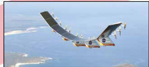
**Sept. 8, 1999:** The Helios Prototype flew for the first time at the Dryden (now Armstrong) Flight Research Center, Edwards, Calif. The Helios Prototype was the fourth and final aircraft developed as part of an evolutionary series of solar- and fuel-cell-system-powered unmanned aerial vehicles. AeroVironment developed the vehicles under NASA's Environmental Research Aircraft and Sensor Technology program.
