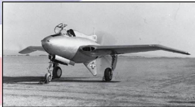
**Sept. 6, 1943:** Northrop's experimental fighter, the XP-56 Black Bullet was trucked to the Muroc lakebed and made its first flight, flown by company test pilot John Myers. The XP-56 was a near-tailless design with a pusher engine driving contra-rotating propellers. It was the first aircraft to be constructed entirely of magnesium.
