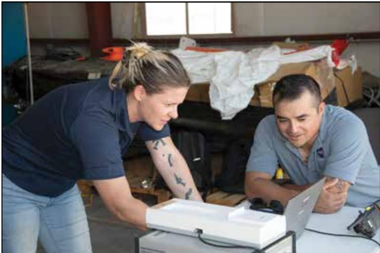
Tegan French and Rocky Garcia are at a weather balloon system's ground station monitoring temperature, humidity, pressure, and winds transmitted from an instrument package on the balloon as it ascends at NASA's Armstrong Flight Research Center at Edwards, Calif.
