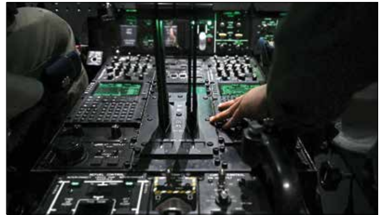
U.S. Air Force Capt. Alex Frazier, 79th Rescue Squadron pilot, sets performance data on an HC-130J Combat King II simulation aircraft during routine training at Davis-Monthan Air Force Base, Arizona, Aug. 9, 2023. The data calculated the speed and distance the aircraft would need for a safe takeoff.
