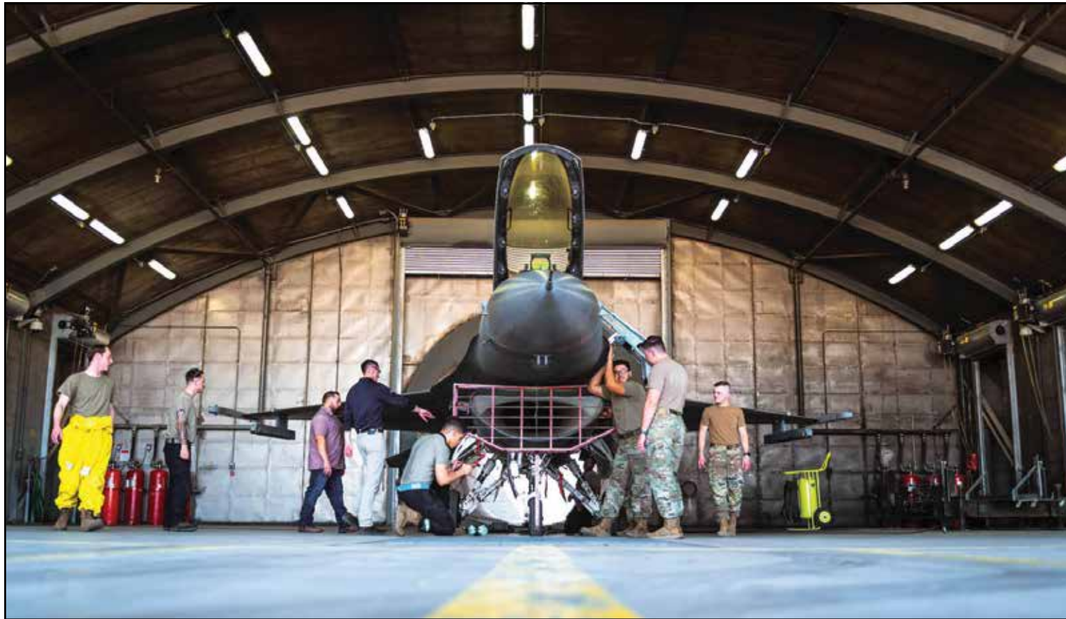
Air Force Engineering Technical Services personnel and U.S. Air Force Airmen assigned to the 56th Fighter Wing, prepare to conduct installed engine operation certification, July 20, 2023, at Luke Air Force Base, Arizona. Under the direction of AFETS personnel, the maintainers performed engine startup and shutdown procedures, engine idle, intermediate and maximum operation, and a review of all emergency procedures for their initial engine operation certification.
