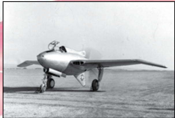
Sept. 6, 1943: Northrop's experimental fighter, the XP-56 Black Bullet was trucked to the Muroc lakebed and made its first flight, flown by company test pilot John Myers. The XP-56 was a near-tailless design with a pusher engine driving contra-rotating propellers. It was the first aircraft to be constructed entirely of magnesium.
