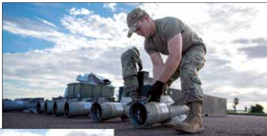
U.S. Air Force Airman 1st Class Eric Mitchell, 56th Equipment Maintenance Squadron munition systems technician, tightens screws on a KMU-572 tail kit, Aug. 11, 2022, at Luke Air Force Base, Arizona. Munition systems technicians are a vital part of the maintenance force that are responsible for ensuring their aircraft are combat-ready.
