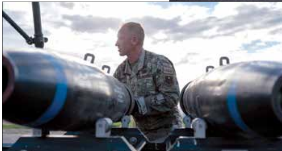
U.S. Air Force Airman 1st Class Eric Mitchell, 56th Equipment Maintenance Squadron munition systems technician, tightens screws on a KMU-572 tail kit, Aug. 11, 2022, at Luke Air Force Base, Arizona. Munition systems technicians are a vital part of the maintenance force that are responsible for ensuring their aircraft are combat-ready.
