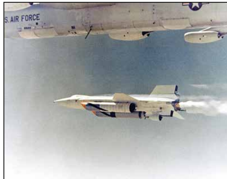
After an ablative coating to protect the craft from high-temperature flight, the X-15 was then covered with a white sealant coat and mounted with additional external fuel tanks.
