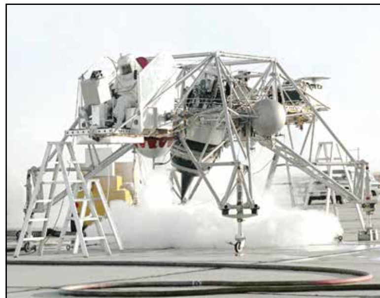
This 1964 photograph shows a ground engine test underway on the Lunar Landing Research Vehicle (LLRV) No. 1.
