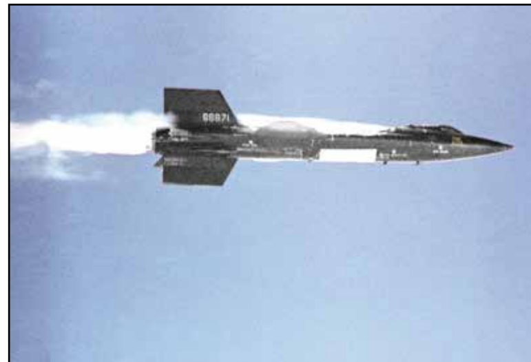
The X-15 No. 2 (56-6671) launches away from the B-52 mothership with its rocket engine ignited.
