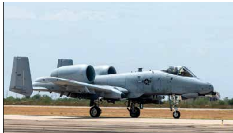
A U.S. Air Force A-10C Thunderbolt II, assigned to the 354th Fighter Generation Squadron, taxis on the flightline at Davis-Monthan Air Force Base, Aug. 23, 2023. The A-10 was designed to provide close air support to friendly ground troops by attacking armored vehicles, tanks, and other enemy ground forces.
