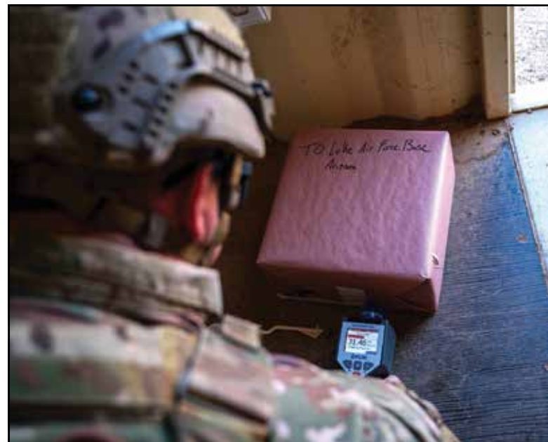
U.S. Air Force Staff Sgt. Zackary Stringer, 56th Civil Engineer Squadron explosive ordnance disposal technician, uses a radiological isotope identification device during training exercise Road RAPTER or Radiological Assistance Program Training for Emergency Response Sept. 7, 2023, at Luke Air Force Base, Arizona. Identification devices are one of several tools used by EOD when assessing the danger represented by a radiological dispersion device.
