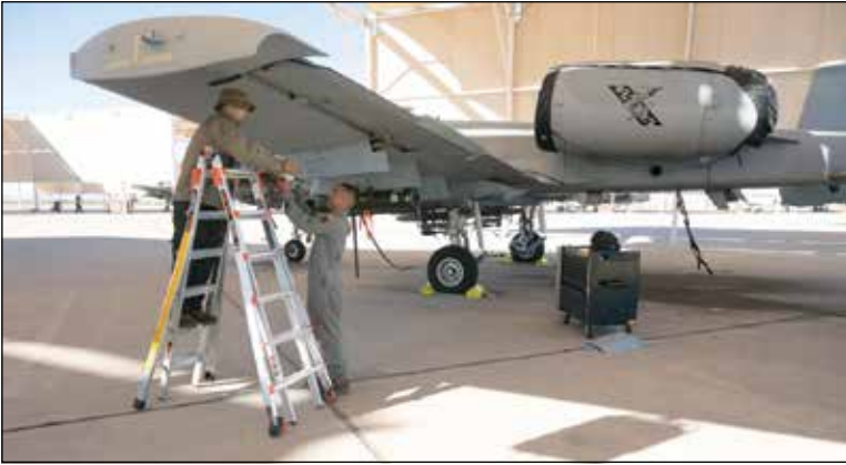
U.S. Air Force Airman 1st Class Max Velez, 357th Fighter Generation Squadron weapons load crew member, and U.S. Air Force Senior Airman Blake Hewitson, 357th Fighter Generation Squadron weapons load crew member, load chaff and flare countermeasures onto an A-10C Thunderbolt II aircraft. The A-10 aircraft was designed to be serviced and operated from bases with limited facilities near battle areas.
