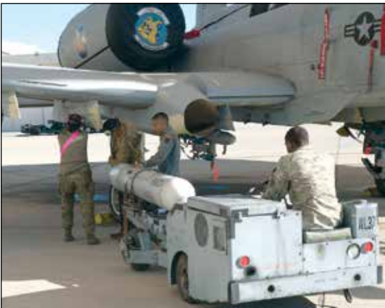
U.S. Air Force Airmen load a missile onto an A-10C Thunderbolt II aircraft at Davis-Monthan Air Force Base. The A-10 aircraft was designed for the close air support mission and has the ability to carry 16,000 pounds of ordinance.
