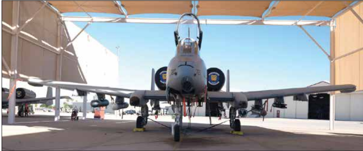
An A-10C Thunderbolt II aircraft is displayed at Davis-Monthan Air Force Base, Arizona, Nov. 9, 2023. The A-10 aircraft's 30mm GAU-8/A Avenger was designed to fire 3,900 rounds per minute and can defeat an array of ground targets, including tanks.
