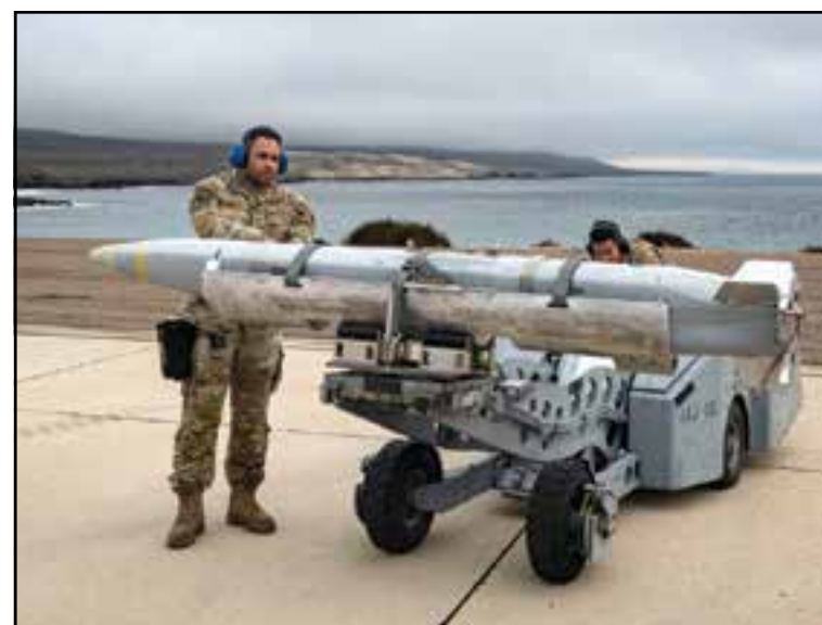
Weapons load crew Airmen, assigned to the 757th Aircraft Maintenance Squadron, Nellis Air Force Base, Nev., maneuver a DATM-160, a training version of the ADM-160 Miniature Air-Launched Decoy during Green Flag-West 23-02 on San Clemente Island, Calif., Nov. 7, 2022.
