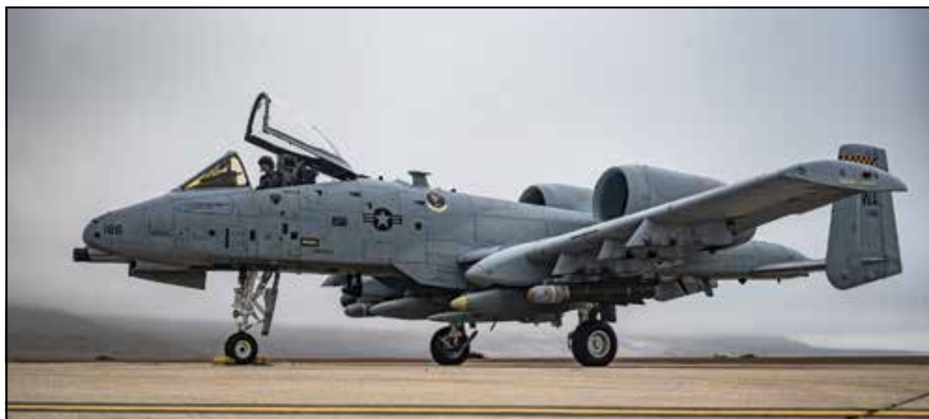
An A-10C Thunderbolt II assigned to the 66th Weapons Squadron, Nellis Air Force Base, Nev., loaded with a DATM-160 training version of the ADM-160 Miniature Air-Launched Decoy, sits on San Clemente Island, California, November 7, 2022.
